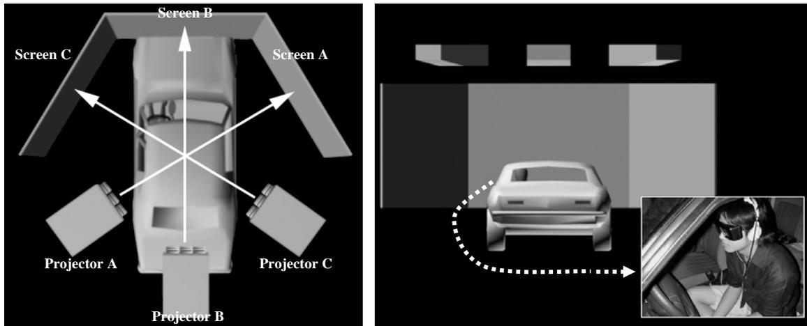
**Figure 2.** Equipment setting. The left figure shows the top view, and the right figure shows the back view of the setting and the close view to the subject's posture in the experiment.
